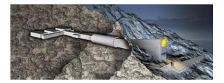
Underground structures offer advantages in terms of preservation of objects or products stored within the structure. For example, food preservation is enhanced by the moderate and constant underground temperature conditions and the ability to maintain a sealed environment.
