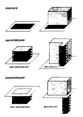
Figure 13. Structural types of parking facilities, categorized by location in relation to the surface.
