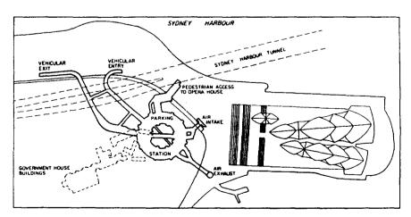
Figure 4. Location plan of the Sydney Opera House Underground Car Park (Source: Pells 1993).
