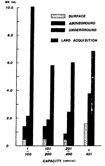
Figure 16. Construction costs of parking facilities.
