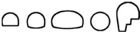
Fig. 1: Typical cross sections in conventional tunnelling
