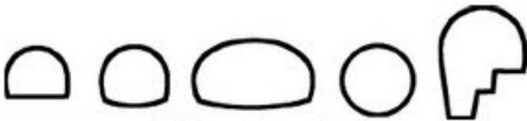
Fig. 1: Typical cross sections in conventional tunneling
