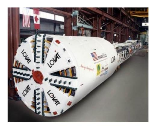
Besides the specific way of supporting the tunnel periphery and face, the specific method of ground excavation is also an important characteristic of shield machines.
