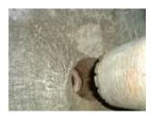
Destructive investigations consist in drilling the lining. They are essential in any case to calibrate non destructive investigations.
