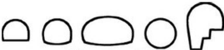
Fig. 1: Typical cross sections in conventional tunneling
