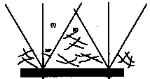
Figure 4.1 - Exemple schematic of liner loading (after Barrett & McCreath, 1995).
